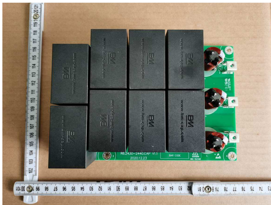
Figure 20. Front view of Capacitance. board
