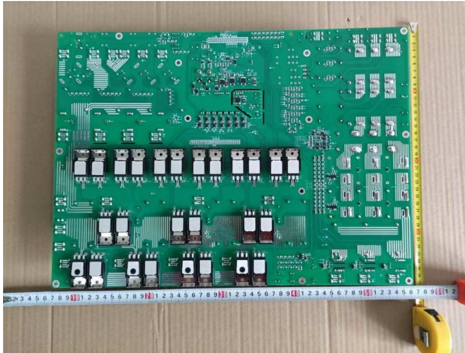
Figure 9. Back view of Main power board for R6-36K-T4-32, R6-40K-T4-32, R6-50K-T4-32, R6-25K-T4-32-LV, R6-30K-T4-32-LV(AC side with varistor)
