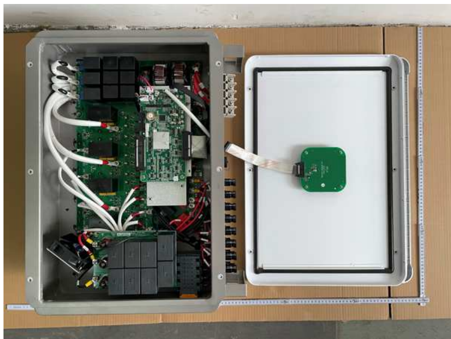
Figure 6. Internal view of R6-36K-T4-32, R6-40K-T4-32, R6-50K-T4-32, R6-25K-T4-32-LV, R6-30K-T4-32-LV
