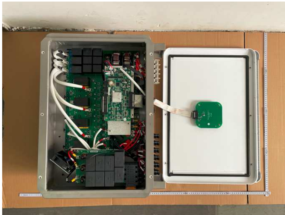
Figure 7. Internal view of R6-25K-T3-32, R6-30K-T3-32, R6-33K-T3-32, R6-36K-T3-32, R6-20K-T3-32-LV
