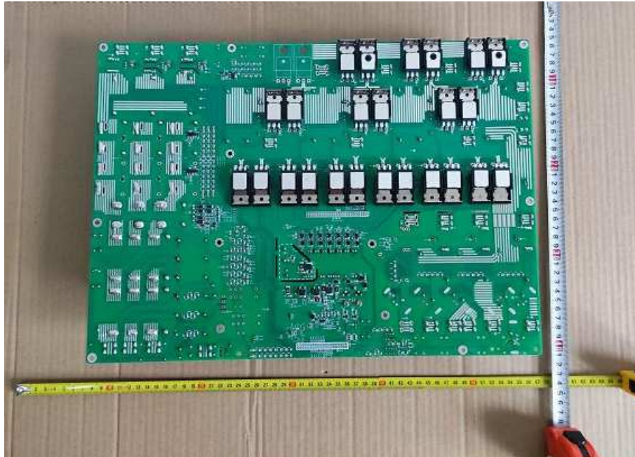
Figure 15. Back view of Main power board for R6-25K-T3-32, R6-30K-T3-32, R6-33K-T3-32, R6-36K-T3-32, R6-20K-T3-32-LV(AC side with Surge Protector version)
