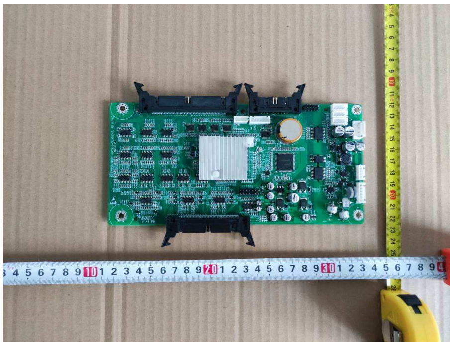
Figure 16. Front view of Control communication board
