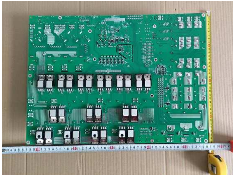
Figure 11. Back view of Main power board for R6-36K-T4-32, R6-40K-T4-32, R6-50K-T4-32, R6-25K-T4-32-LV, R6-30K-T4-32-LV(AC side with Surge Protector version)
