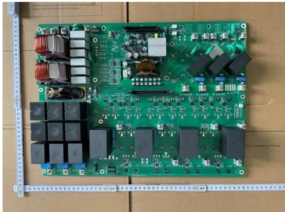
Figure 12. Front view of Main power board for R6-25K-T3-32, R6-30K-T3-32, R6-33K-T3-32, R6-36K-T3-32, R6-20K-T3-32-LV(AC side with varistor)
